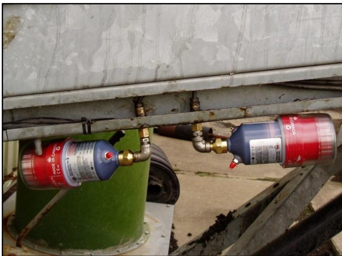
MD125 Ultimate Lubricator fitted to conveyor
